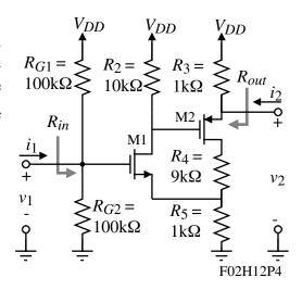
2.) A feedback amplifier is shown. Use the methods of feedback analysis to find the numerical values of  $v_2/v_1$ ,  $v_1/i_1$ , and  $v_2/i_2$ . Assume that all transistors are matched and that  $g_m = 1$ mS, and  $r_{ds} = \infty$ .
