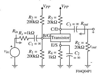
c.) In your own words tell why the small-signal voltage gain of the BJT CE amplifier is greater (roughly x10) than the small-signal voltage gain of the NMOS CS amplifier when the currents are the same and the external circuit is the same.
