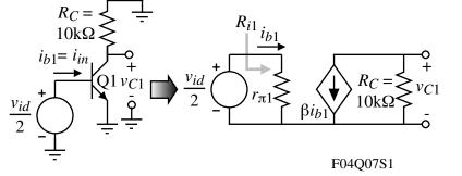
$$\frac{v_{C1}}{v_{id}} = \frac{1}{2} \frac{v_{C1}}{v_{id}/2} = \frac{1}{2} \left( \frac{v_{C1}}{i_{b1}} \right) \left( \frac{i_{b1}}{v_{id}/2} \right) = \frac{1}{2} \left( \frac{v_{C1}}{i_{b1}} \right) \left( \frac{1}{R_{i1}} \right) = \frac{-\beta R_C}{2R_{i1}} = \frac{-100 \cdot 10 \text{k}\Omega}{2 \cdot 5 \text{k}\Omega} = \frac{-100 \text{ V/V}}{2 \cdot 5 \text{k}\Omega}$$
