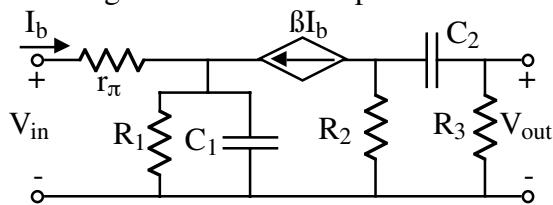
$$\frac{V_{\text{out}}}{V_{\text{in}}} = \left( \frac{V_{\text{out}}}{I_b} \right) \left( \frac{I_b}{V_{\text{in}}} \right) = \left( \frac{-\beta R_2 R_3}{R_2 + R_3 + \frac{1}{sC_2}} \right) \left( \frac{1}{r_\pi + (1+\beta) \left( \frac{R/sC_1}{R_1 + \frac{1}{sC_1}} \right)} \right)$$
