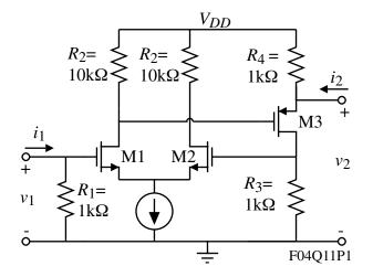
The circuit for calculating the small-signal open-loop gain is,
