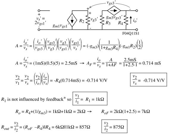
\* The reason for this is that the input variable is  $v_s$  and the resistor,  $R_1$ , in parallel with  $v_s$  does not influence the circuit so the input resistance without feedback is  $\infty$ .
