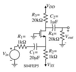
Because the capacitors are independent, probably the best way to work this problem is by superposition (open-circuit time constants). Therefore, C:
