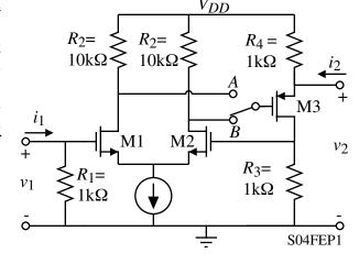
(b.) This feedback circuit is series-series. The units of A are A/V and the units of  $\beta$  are V/A.
