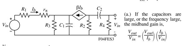
$$\frac{V_{out}}{V_{in}} = \left(\frac{V_{out}}{I_b}\right) \left(\frac{I_b}{V_{in}}\right)$$
