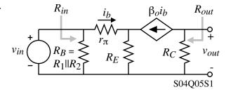
$(R_B = R_1 || R_2 \text{ is not part of this because it is in parallel with } v_{in} \text{ and is not a part of } R_{in}.)$
