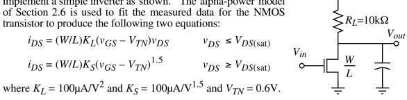
a.) Derive the expression for  $V_{DS(sat)}$  assuming the model above.
