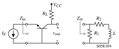
*L* in terms of the parameters of the BJT small signal model ( $r_b$ ,  $r_\pi$ ,  $C_\pi$ , and  $\beta_o$ ). Ignore  $r_o$  and assume that  $R_1 > R_2$ .
