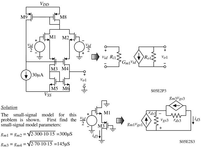
$r_{ds1} = r_{ds2} = r_{ds5} = r_{ds6} = 50/15 \mu A = 3.33 M\Omega$  and  $r_{ds3} = r_{ds4} = 25/15 \mu A = 1.67 M\Omega$ Summing currents:
