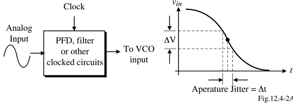
If we assume that  $v_{in}(t) = V_p \sin \omega t$ , then the maximum slope is equal to  $\omega V_p$ .
