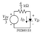
(b.) With  $V_{IN}$  = -10V, we know the diode is reverse biased. Therefore replacing it with an open-circuit gives,
