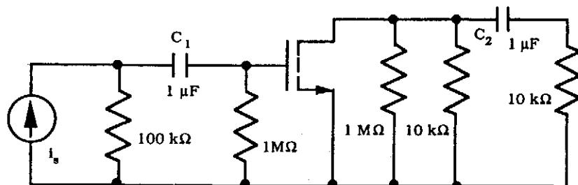
$$\omega_1 = \frac{1}{10^{-6}(100\text{k}\Omega + 1\text{M}\Omega)} = 0.909 \frac{\text{rad}}{\text{s}} \quad | \quad \omega_2 = \frac{1}{10^{-6}(10\text{k}\Omega + 25\text{k}\Omega || 10\text{k}\Omega || 1\text{M}\Omega)} = 58.5 \frac{\text{rad}}{\text{s}}$$
