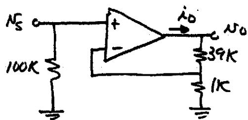
$$N_o = \frac{R_2 + R_1}{R_1} N_s = 40 N_s$$
