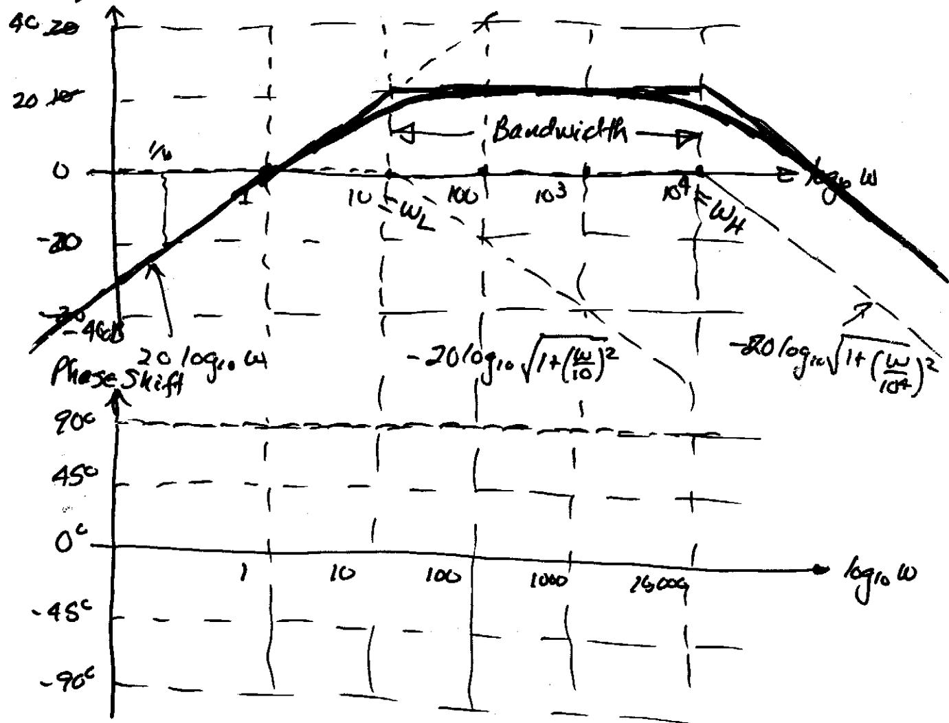
$$\text{Arg}[A_v(j\omega)] = \pm 180^\circ + 90^\circ - \tan^{-1}\left(\frac{\omega}{10}\right) - \tan^{-1}\left(\frac{\omega}{10^4}\right)$$
