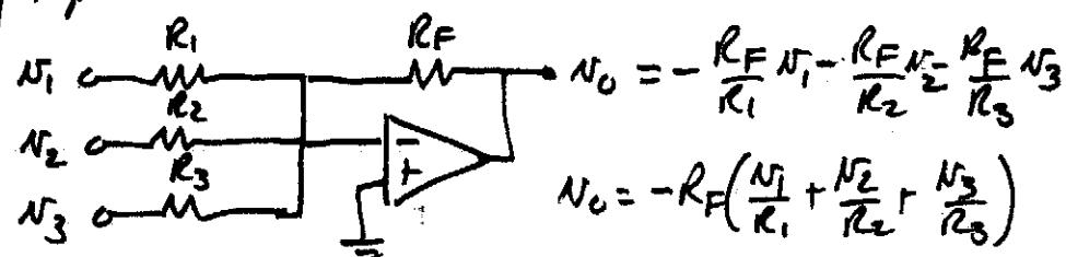
$$N_o = -R_F \left( \frac{N_1}{R_1} + \frac{N_2}{R_2} + \frac{N_3}{R_3} \right)$$
