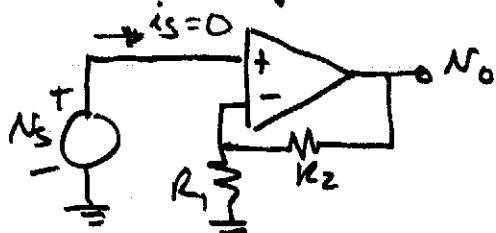
$$N_+ = N_s \quad \& \quad N_- = N_o \frac{R_1}{R_1 + R_2}$$
