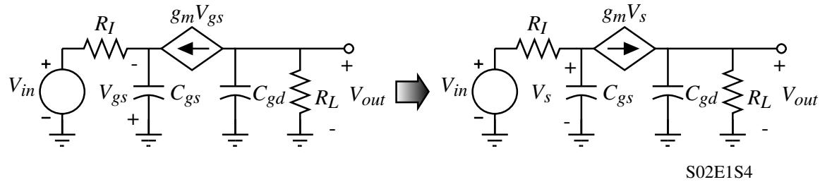
$$V_{out} = g_m Z_L V_s \quad \text{where} \quad Z_L = \frac{1}{s R_L C_{gd} + 1} \quad \text{and} \quad \frac{V_{in} - V_s}{R_I} = g_m V_s + s C_{gs} V_s$$
