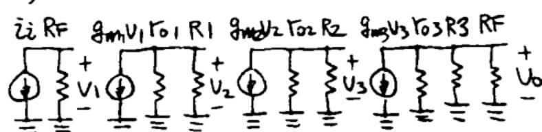
$$A = \frac{U_o}{i_i} |_{f=0} = R_F (-g_m r_{o1} || R_1) (-g_m r_{o2} || R_2) (-g_m r_{o3} || R_3) R_F \\ (-g_m r_{o3} || R_3 || R_F)$$
