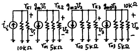
$$r_{\pi 1} = r_{\pi 2} = r_{\pi 3} = \frac{\beta}{g_m} = 5.2 \text{ k}\Omega$$
