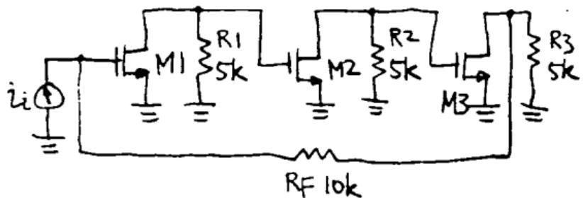
$$g_m = \sqrt{2k'W} I_D = \sqrt{2 \times 60 \times 10^{-6} \times 100 \times 10^{-3}} \\ = 3.5 \times 10^{-3} \text{ A/V}$$
