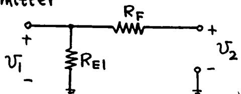
$$f = h_{12} f = \frac{V_i}{V_o} = \frac{R_{E1}}{R_{E1} + R_F}$$
