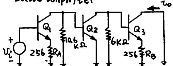
$$R_{S1} \parallel (R_F + R_{E2}) = 290 \parallel 2.19K = 256\Omega$$
